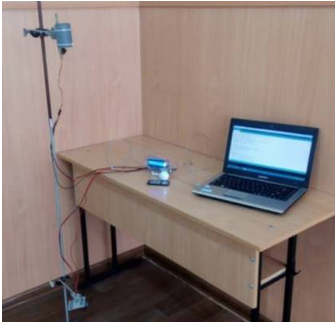
Figure 6: Installation for the acceleration of the accelerated fall.
